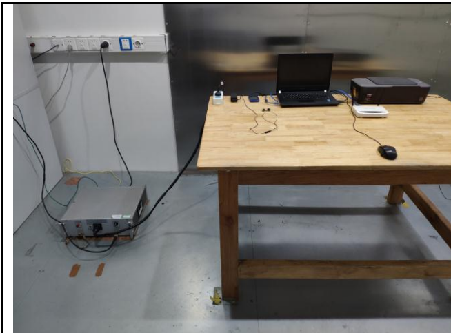
Conducted Emissions Test Setup – Front View
