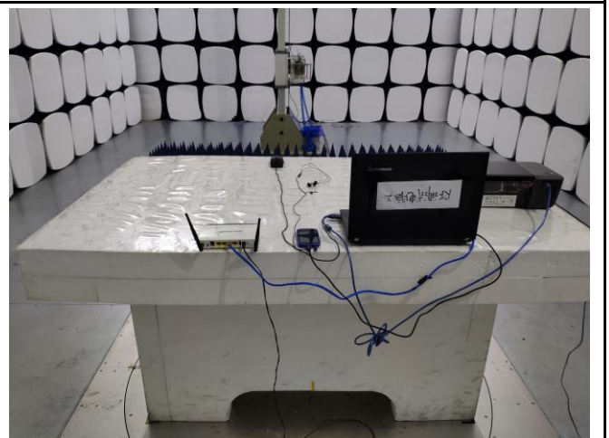
Radiated Emissions Test Setup Above 1GHz
