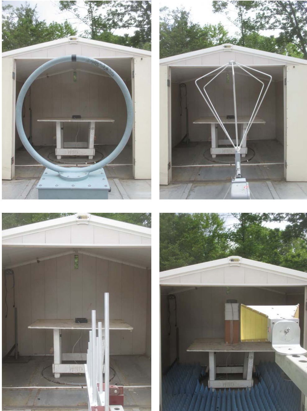
Figure 3.2 Radiated Configuration Test Setup
