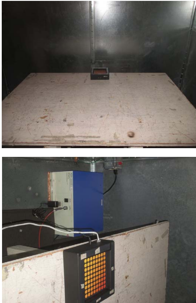
Fig. 3.3 Conducted Emission Test Setup
