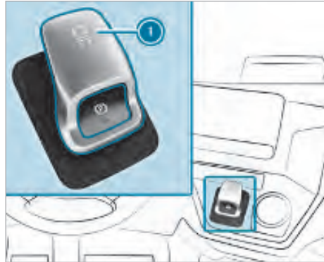
Electric independent trailer brake lever
