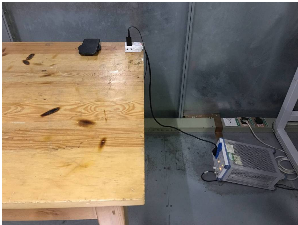
Conducted Emission-AC adapter charge mode
