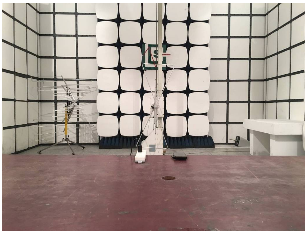
Radiated Emission below 1GHz-AC adapter charge mode
