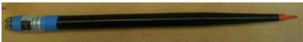
Figure 1 – MVG COMOSAR Dosimetric E-field Dipole
