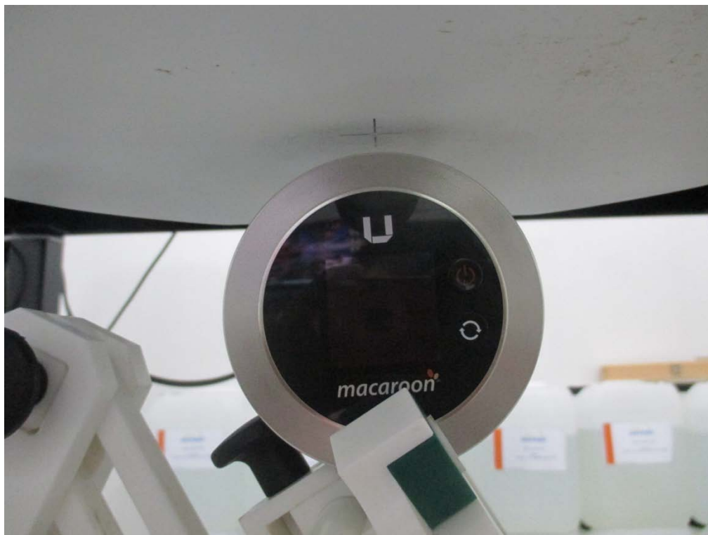
Body top side(separation distance is 5mm)
