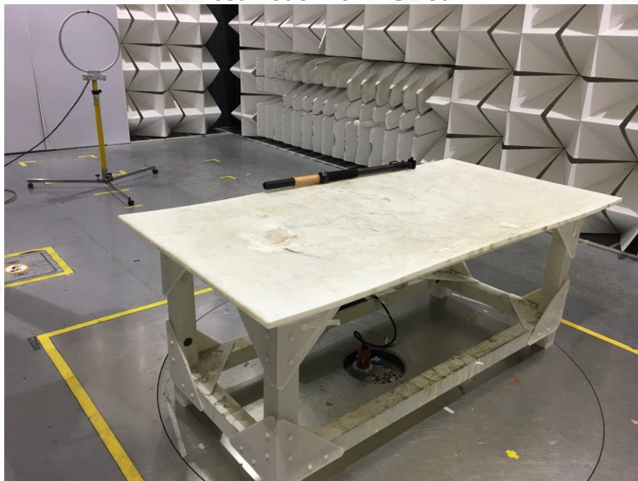
Radiated spurious emission Test Setup-1(Below 30MHz)
