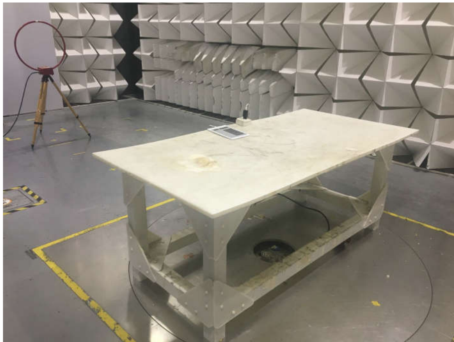
Radiated spurious emission Test Setup-1(Below 30MHz)
