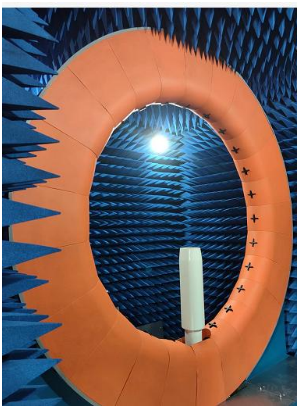
24 probe microwave anechoic chamber test equipment
