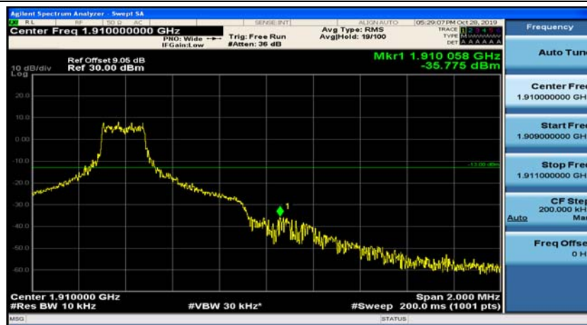
(Channel Bandwidth: 1.4 MHz)_HCH_16QAM_1RB#5
