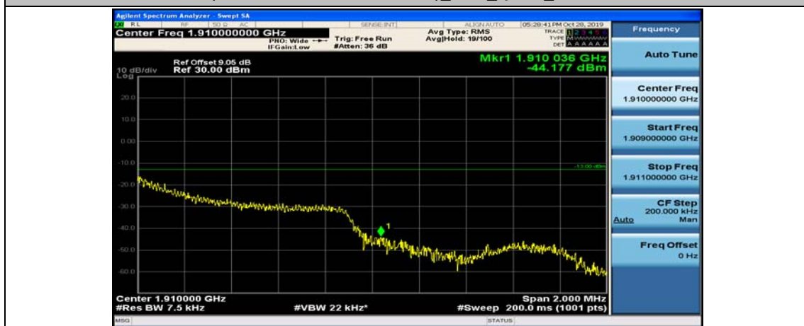
(Channel Bandwidth: 1.4 MHz)_HCH_QPSK_1RB#3
