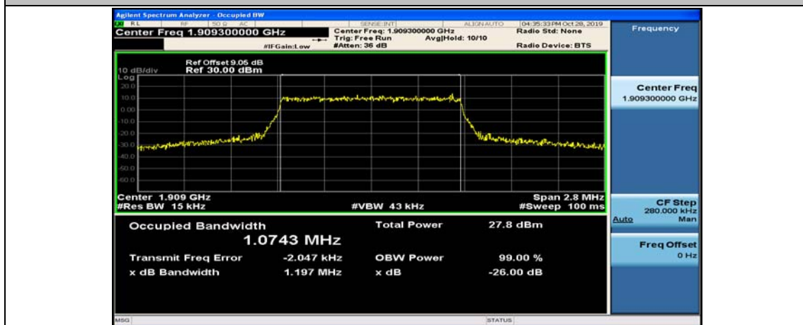
(Channel Bandwidth: 1.4 MHz)_HCH_QPSK_6RB#0
