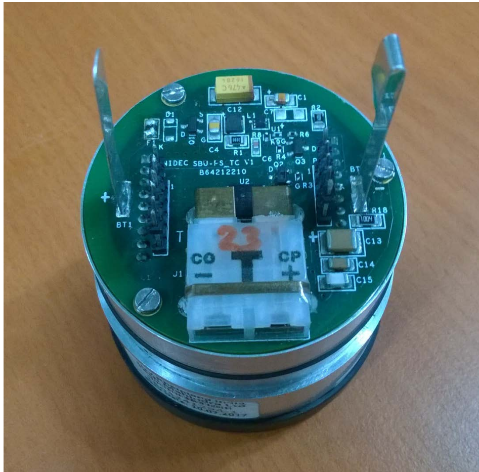
RF Module PCB removed
