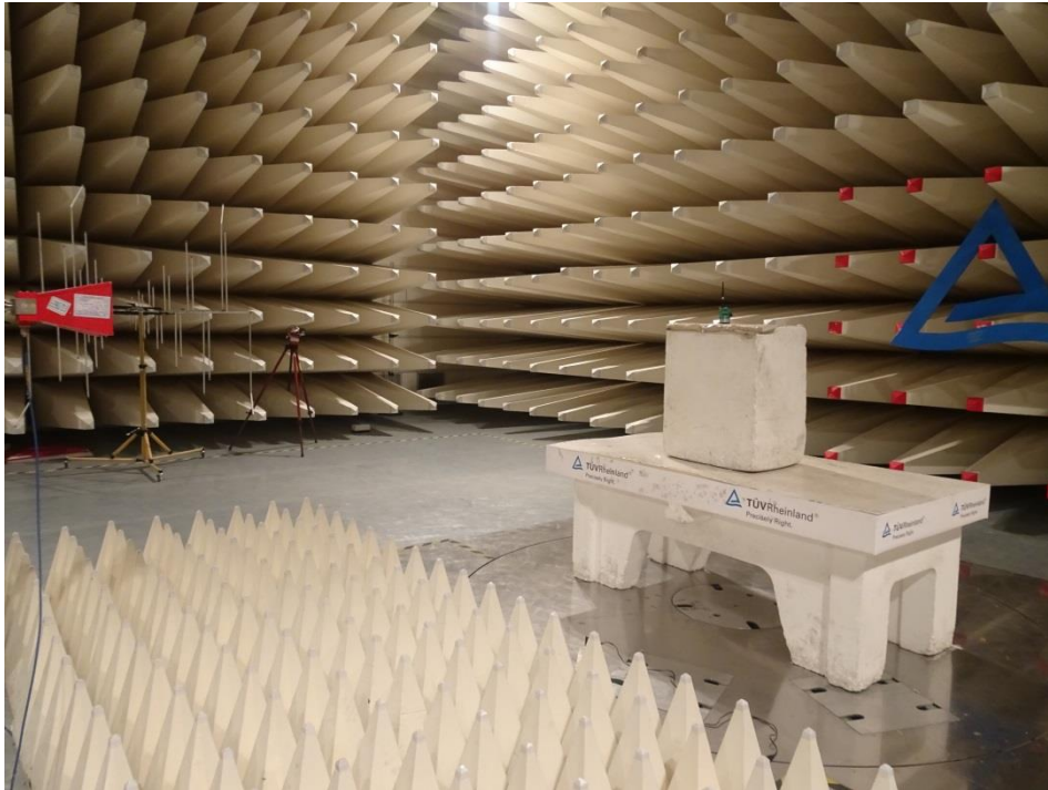
Vertical Polarization Setup Photo - 1 GHz – 18 GHz
