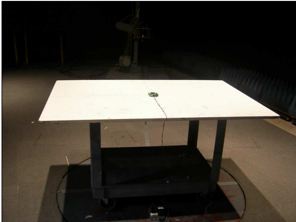
Figure 3: Radiated Emissions – Chip Antenna – Rear View
