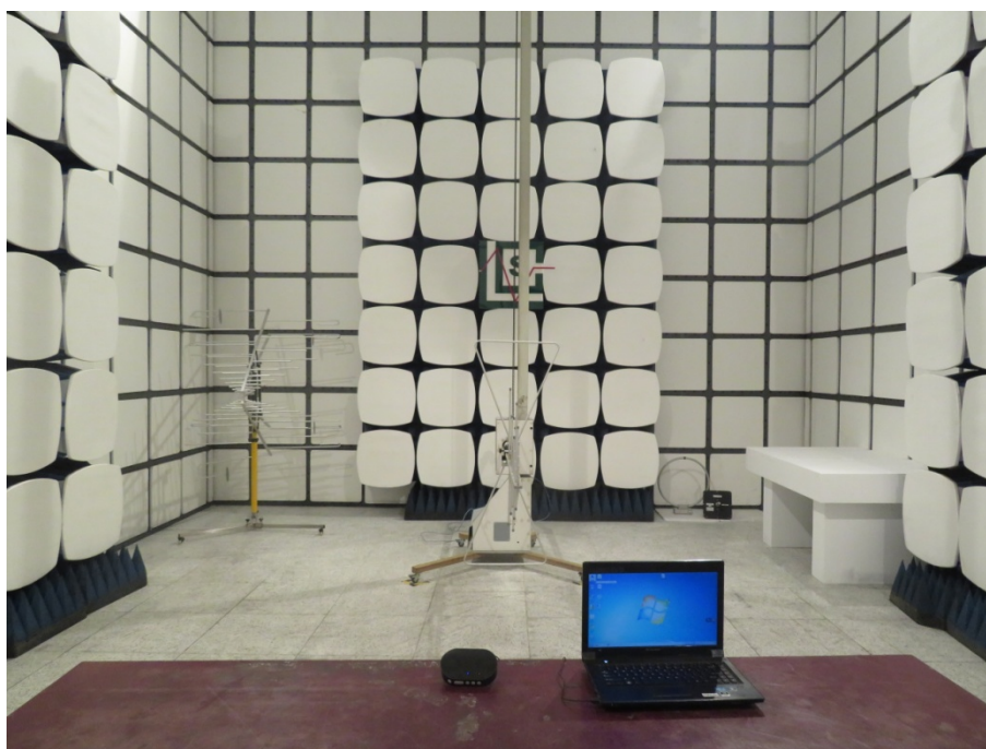
RADIATED EMISSION TEST SETUP (30 MHz to 1 GHz) FROM 1M-HEIGHT TEST TABLE
