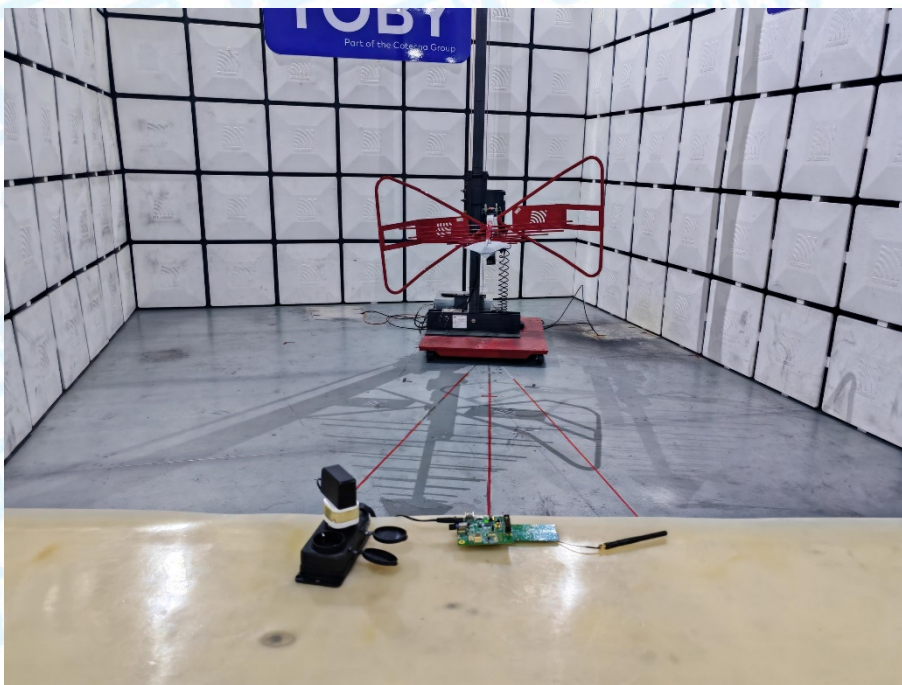
Photo of Setup for Radiated Emission (30MHz~1GHz)
