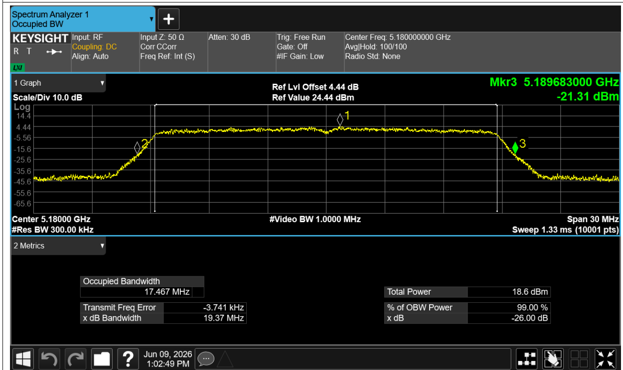
-26dB Bandwidth NVNT n20 5200MHz Ant1
