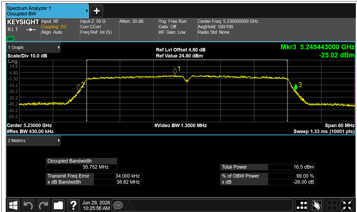
-26dB Bandwidth NVNT ac40 5230MHz Ant2
