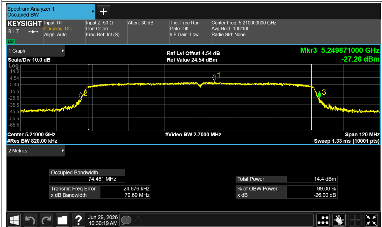
-26dB Bandwidth NVNT n20 5180MHz Ant1
