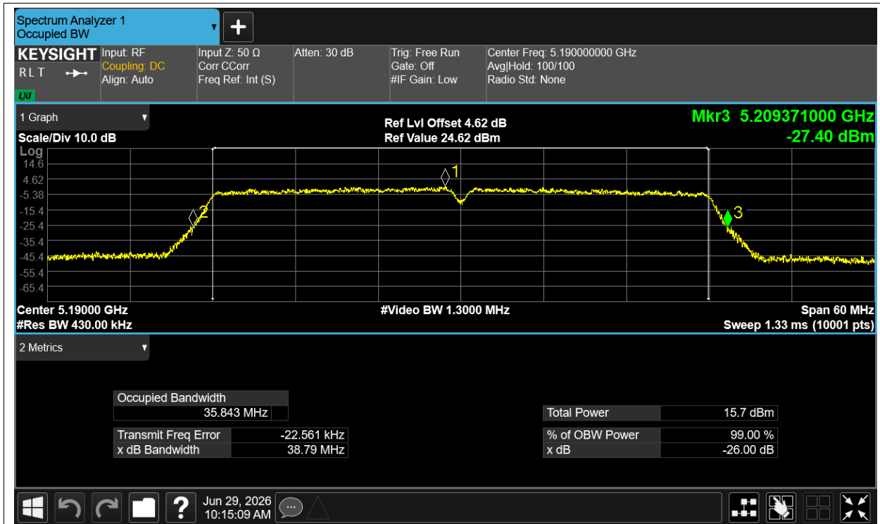
-26dB Bandwidth NVNT n40 5190MHz Ant2
