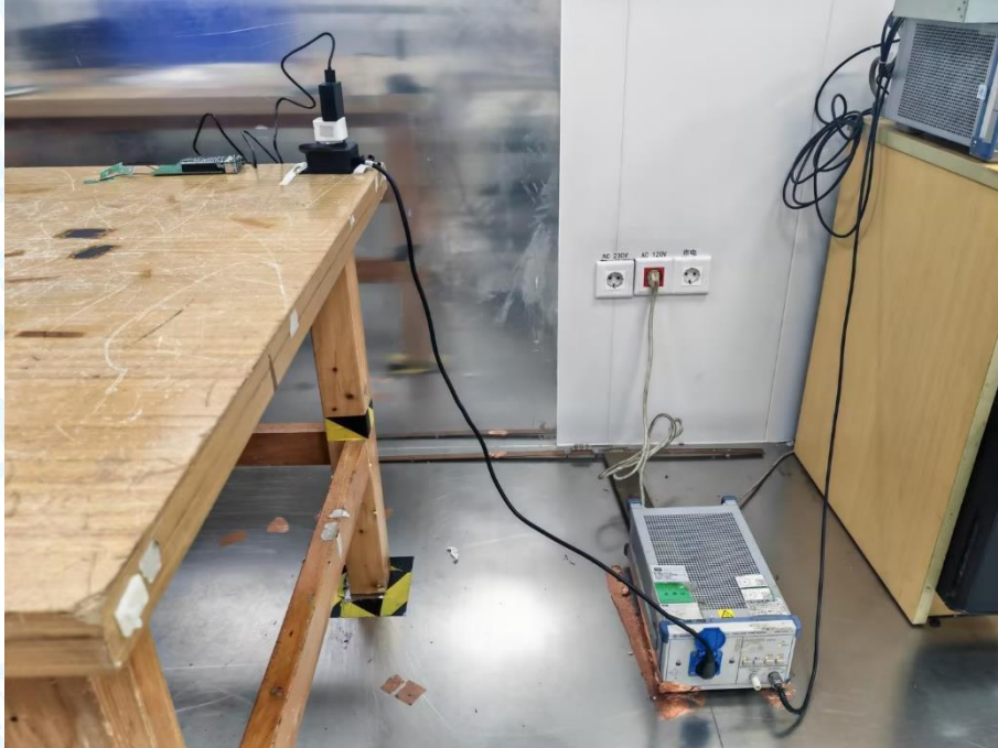
Photo of Setup for Radiated Emission (30MHz~1GHz)
