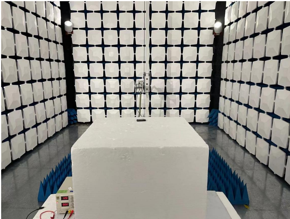
Above 1GHz for radiated emission test setup
