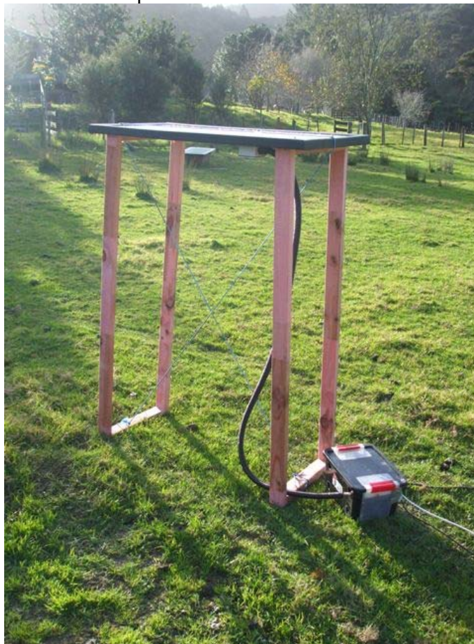
Horizontal panel antenna 1 attached to Master
