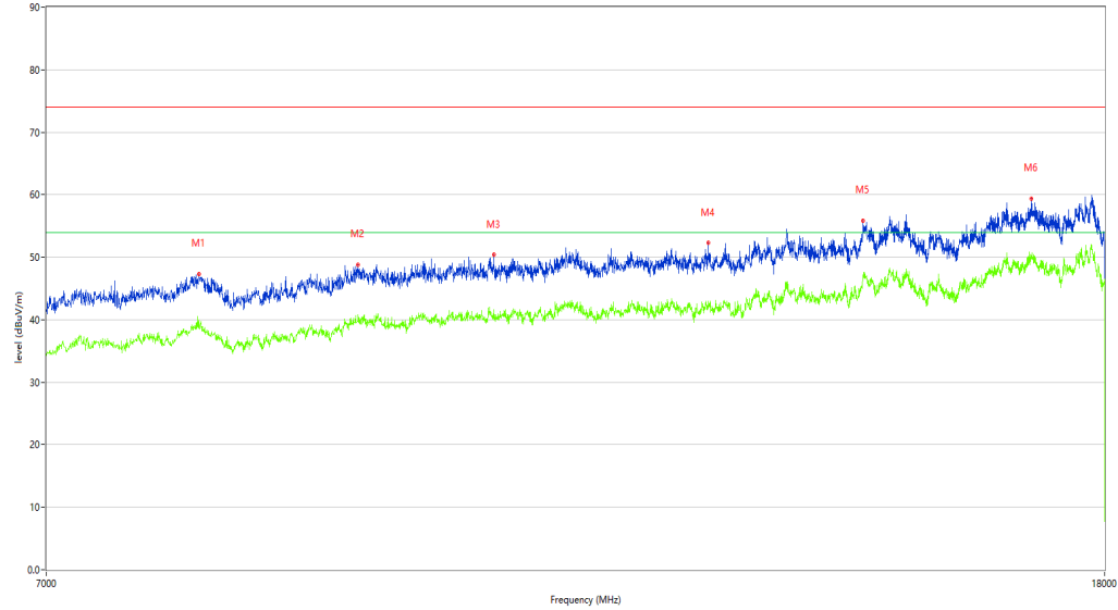
REmission Test case_FCC_Part 15C_FCC 15.247_7GHz-18GHz
