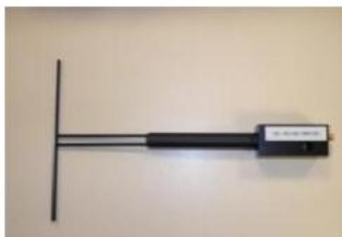
Figure 1 – Satimo COMOSAR Validation Dipole
