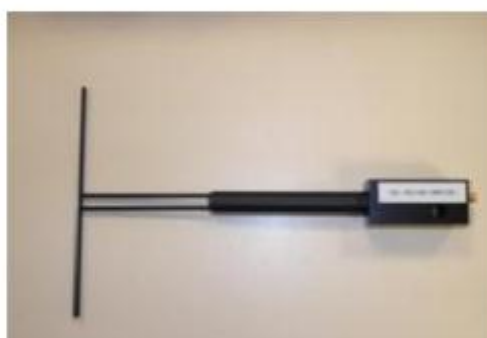
Figure 1 – Satimo COMOSAR Validation Dipole
