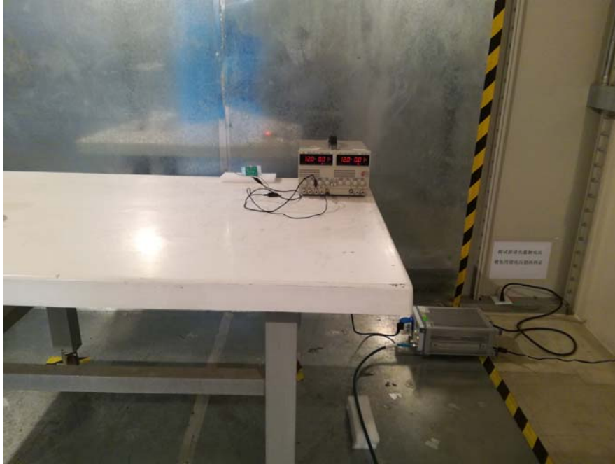
Conducted Emissions (Side View)
