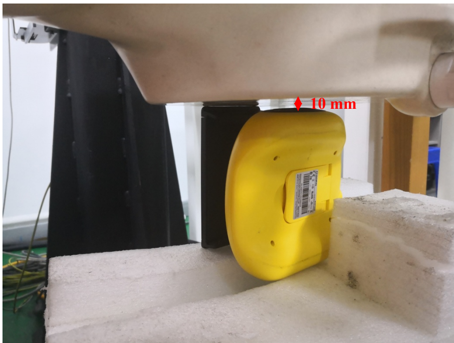
Close to Body Right Setup Photo (10mm)
