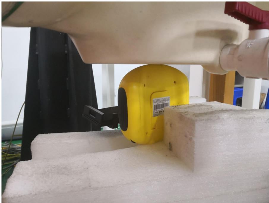
Handheld Bottom Setup Photo (0mm)
