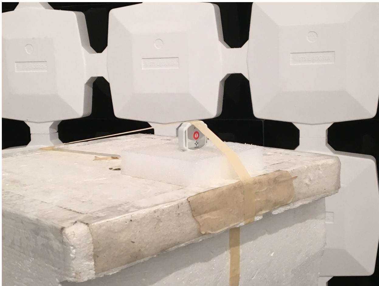
Figure 4- EUT on Raised Block for above 1 GHz Testing
