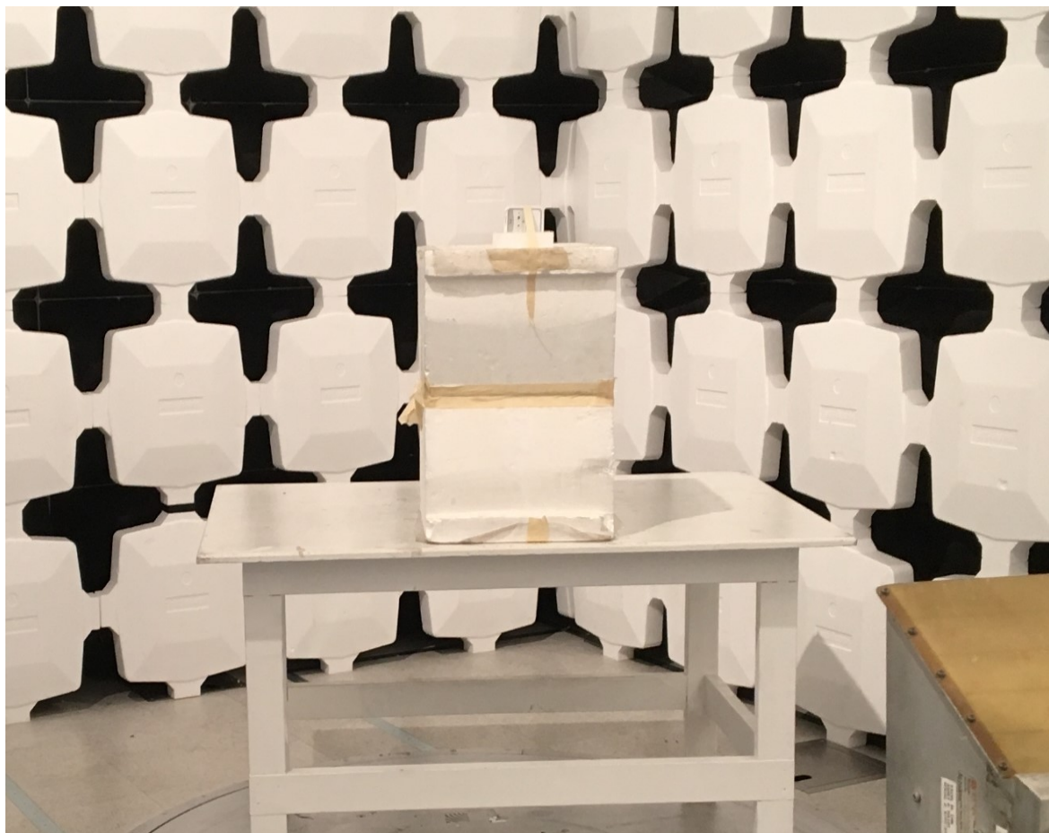
Figure 4. EUT on Raised Block for Above 1 GHz Testing
