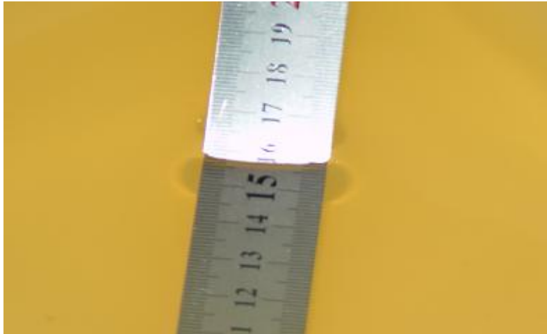
Liquid depth for SAR Measurement
