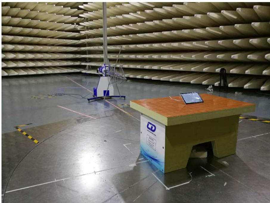
Spurious Radiated Emissions Test setup (30MHz~1GHz)
