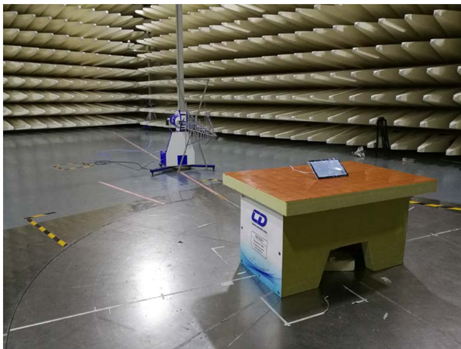
Spurious Radiated Emissions Test setup (30MHz~1GHz)
