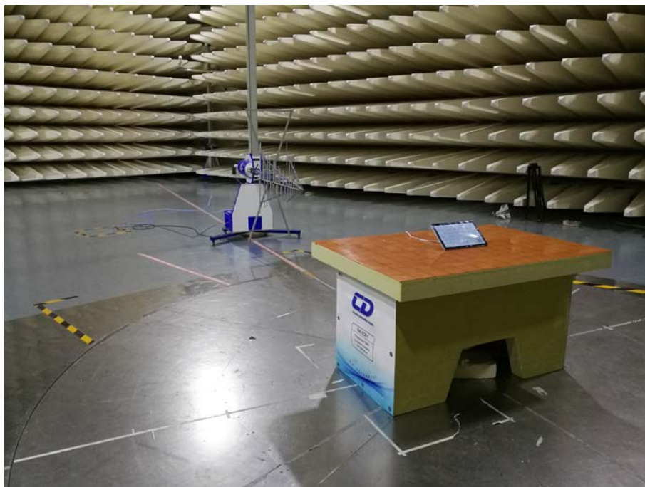
Spurious Radiated Emissions Test setup (30MHz~1GHz)
