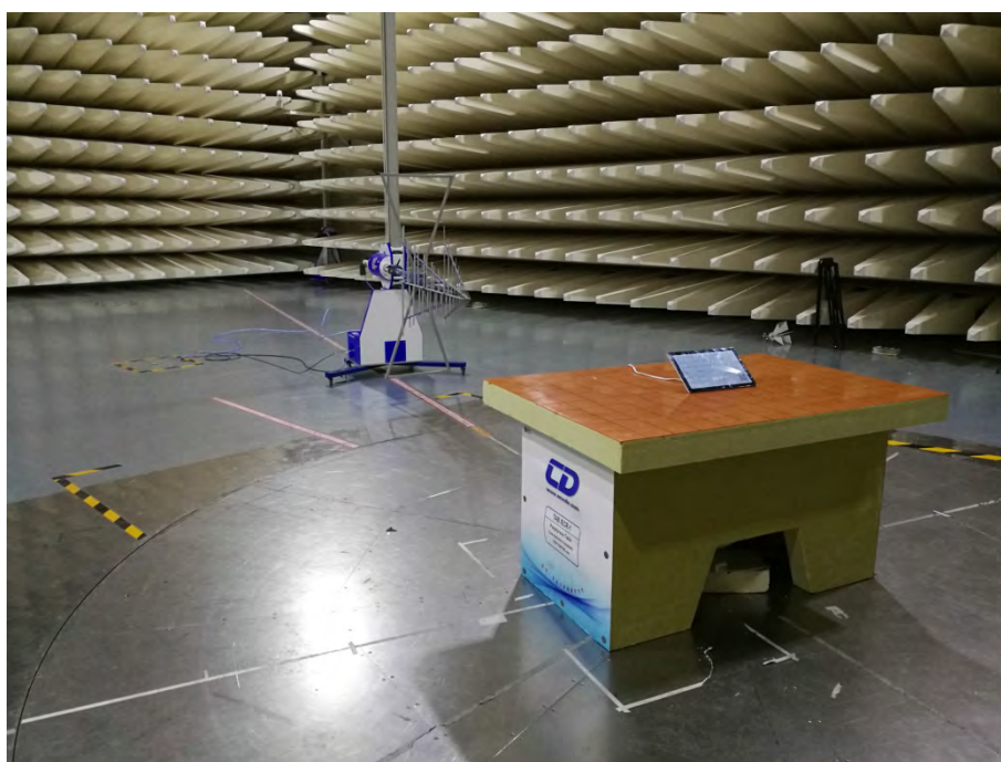
Spurious Radiated Emissions Test setup (30MHz~1GHz)
