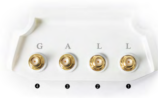
Figure 1.2: Antenna connectors of MX1901/2 Gateway.
