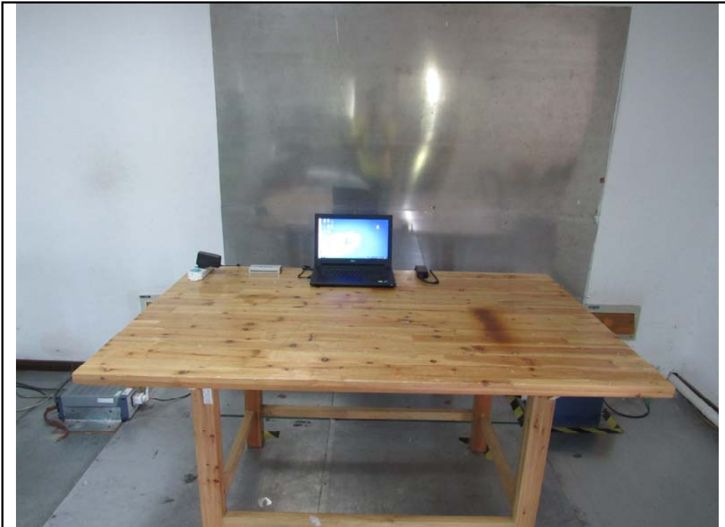
Conducted Emissions Test Setup Front View
