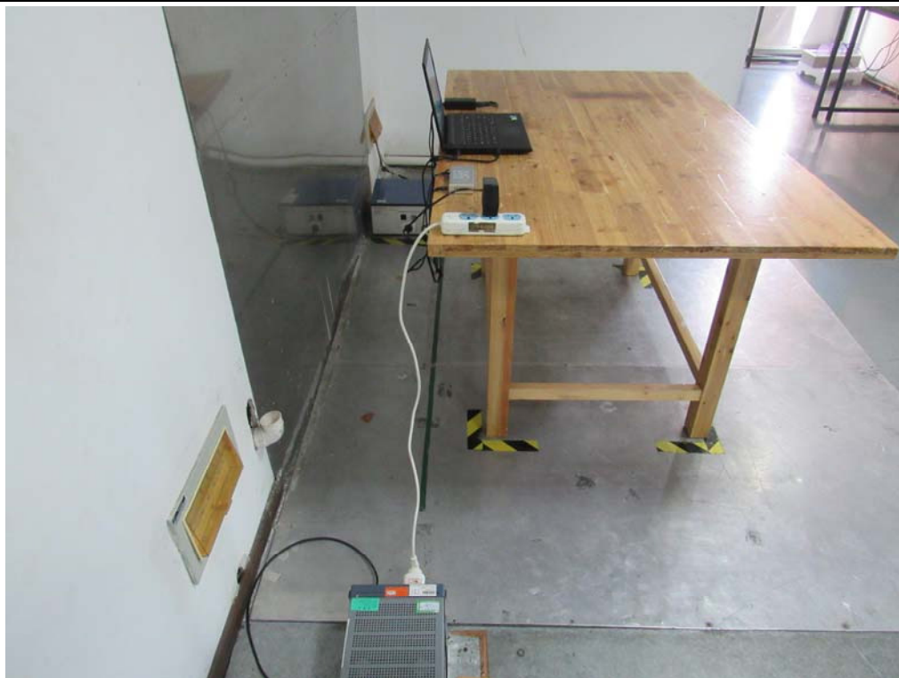
Conducted Emissions Test Setup Side View
