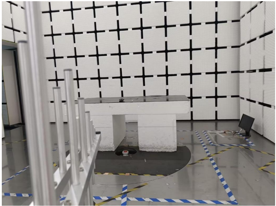
Radiation Emission Test Setup (30MHz to 1GHz)
