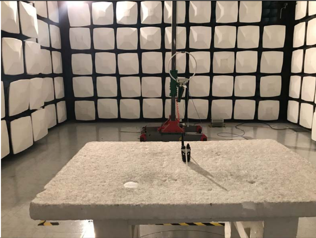
Radiated emission Test Setup (Below 30 MHz)
