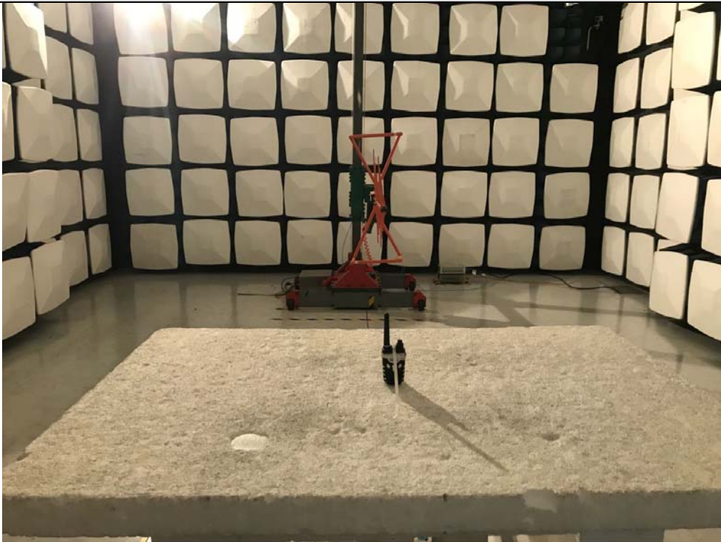
Radiated emission Test Setup (30 MHz~1 GHz)
