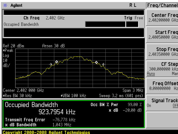
20dB Bandwidth plot on channel 39 (1Mbps)
