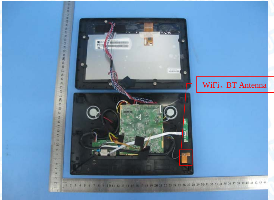
Photo 9 Internal of EUT
