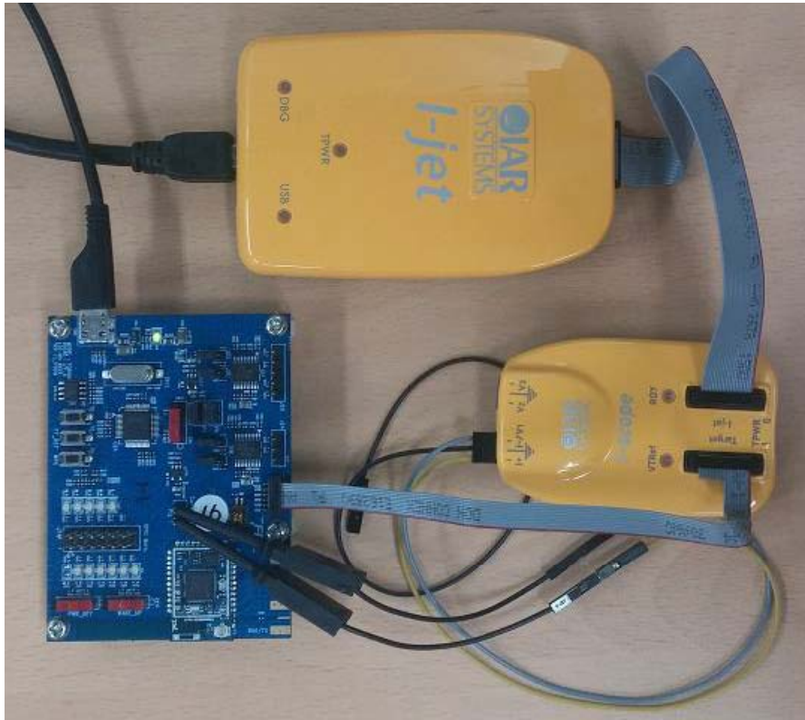
Figure 7. Current Measurement Environment with IAR I-scope
