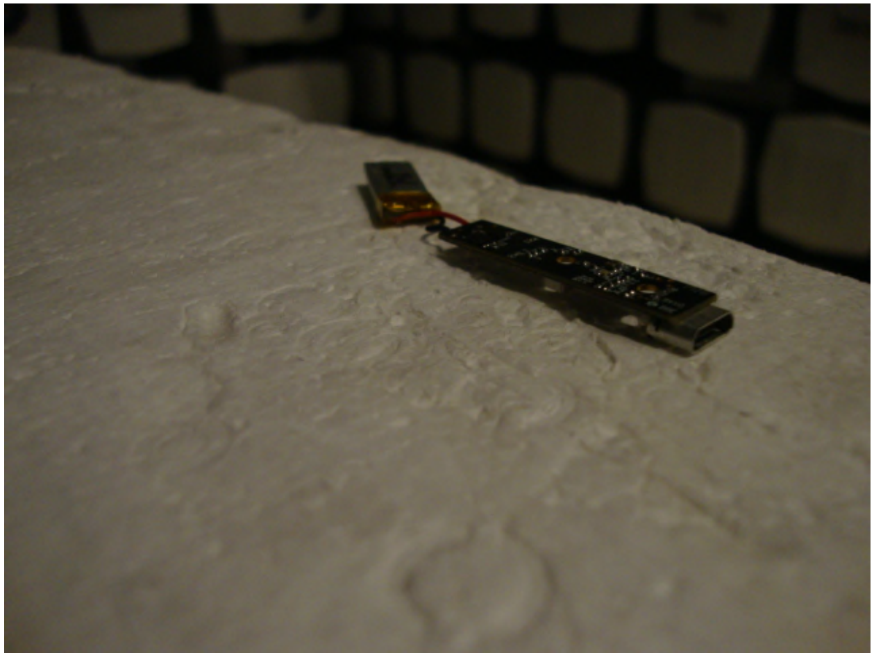
Radiated Emissions Test Setup
