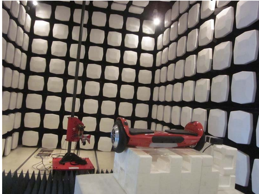
Measurement of Radiated Emission Test Set Up
