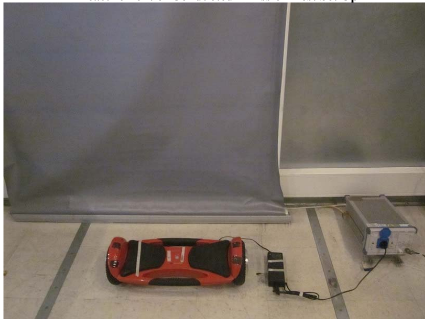
Measurement of Conducted Emission Test Set Up
