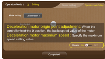
Motor setting Fine tune settings of a selected motor : Steering angle, origin point, speed etc.
