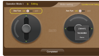
Zero Turn Function When the control slide touch is released, it enables the slide to return to its original position
