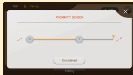
When a sensor value is in the orange area, saved motion is replayed.
