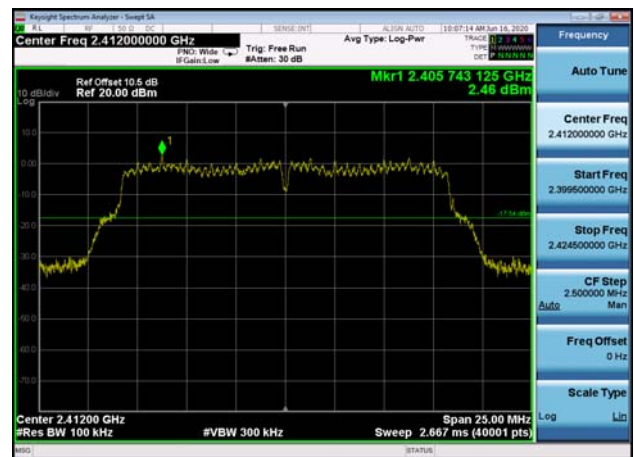
,Plot 1,Reference Level-802.11g ,2462MHz
