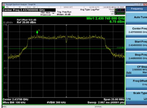
,Plot 1,Reference Level-802.11g ,2437MHz
