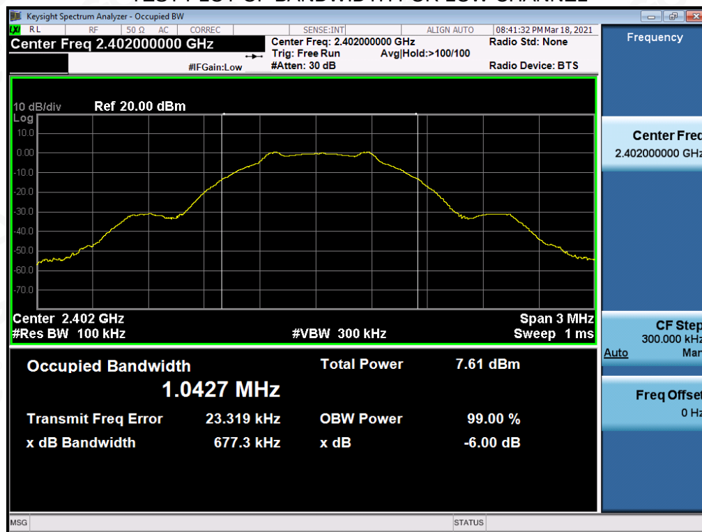
TEST PLOT OF BANDWIDTH FOR LOW CHANNEL
