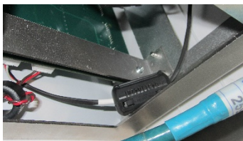
One Ferrite on LED Cable PN: 0431164281
