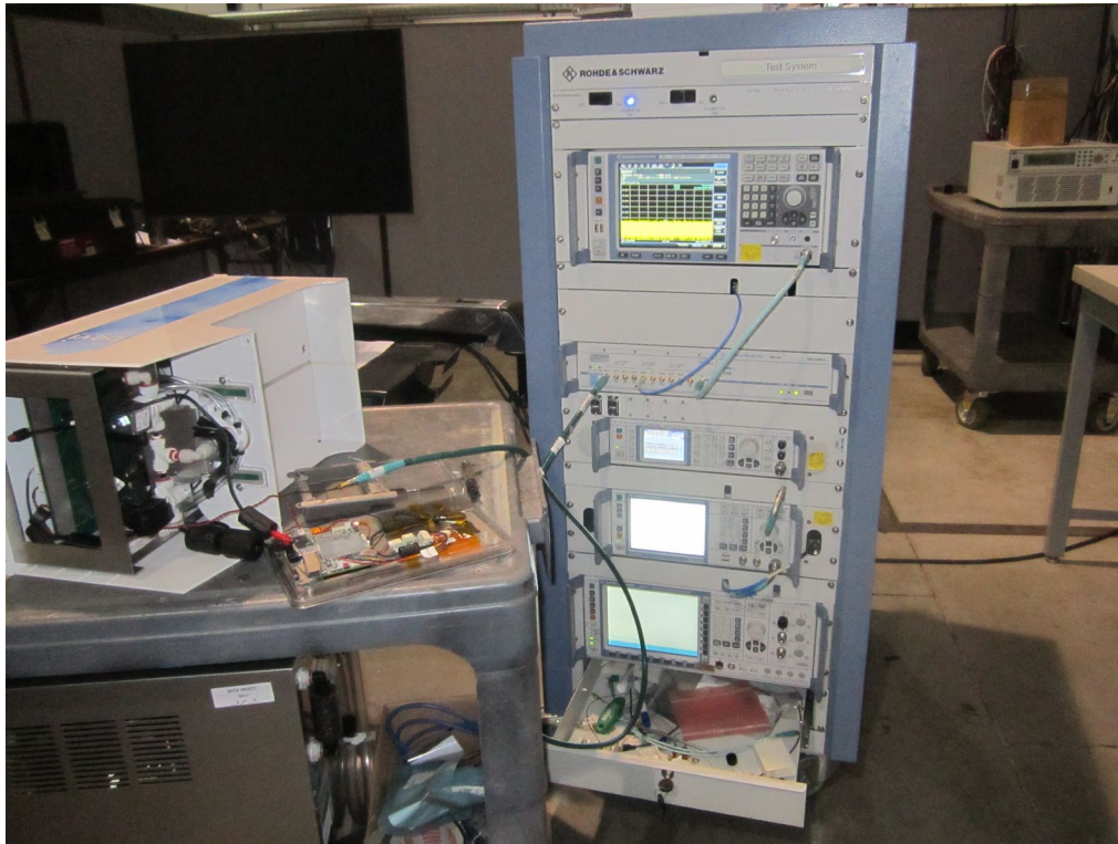
Conducted Antenna port Measurement setup
