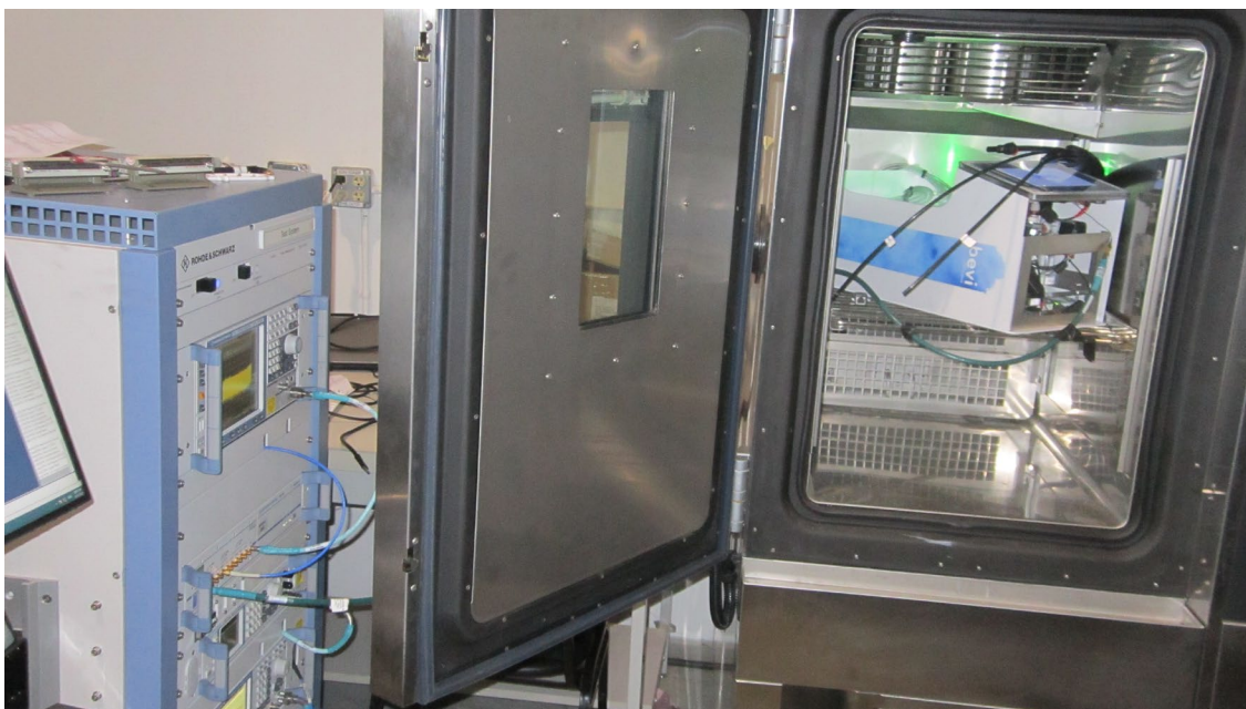
Frequency stability setup, 1
