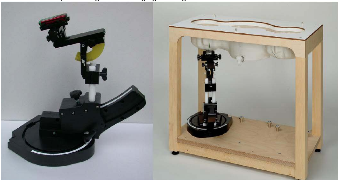
Device holder supplied by SPEAG
