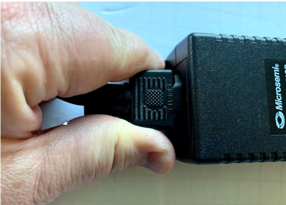
Figure 11: Connecting mains cable to power brick
