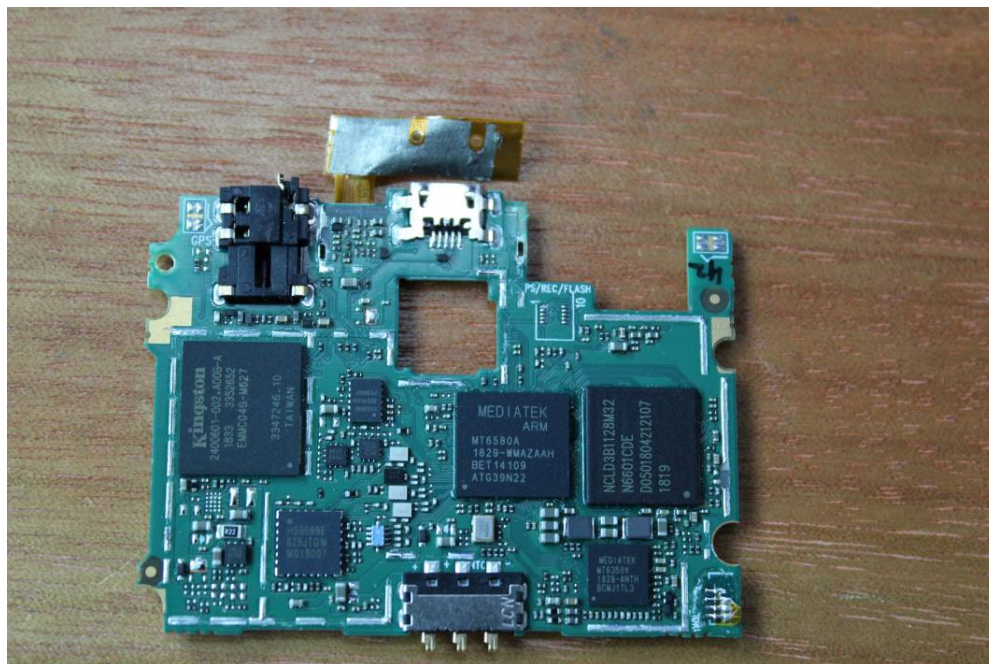
EUT – Main Chip View
