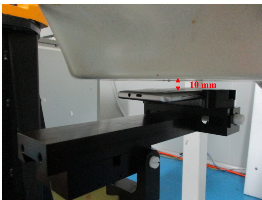
Body (Worn) Back Setup Photo(10mm)
