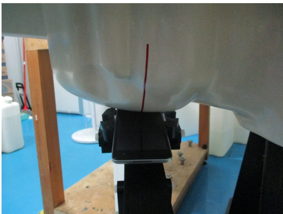
Body (Worn) Back Setup Photo(10mm)
