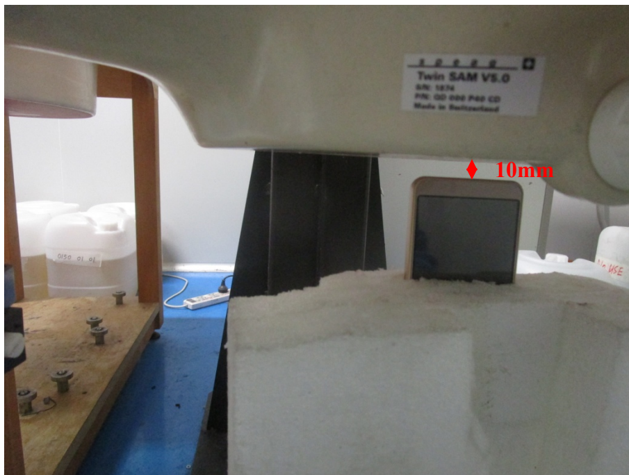
Body Bottom Setup Photo(10mm)
