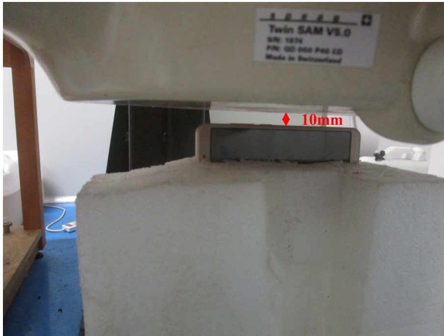
Body Bottom Setup Photo(10mm)
