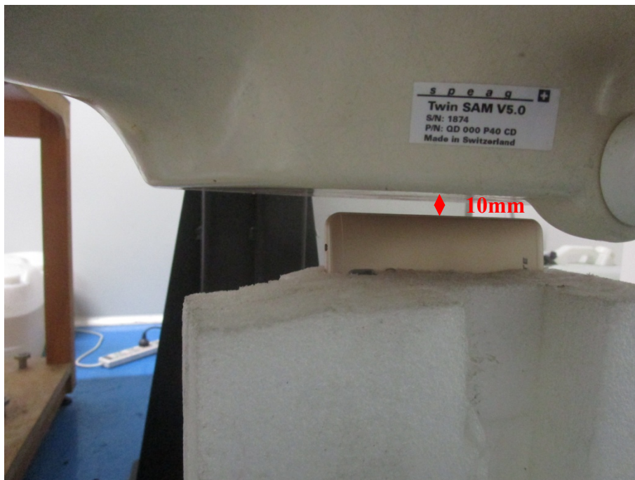
Body Left Setup Photo(10mm)
