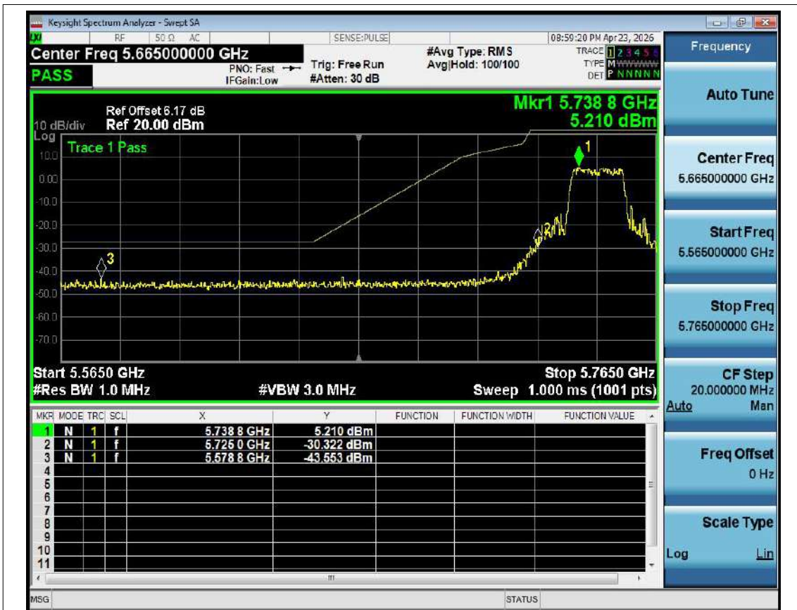
Band Edge NVNT n20 5745MHz Low Ant1
