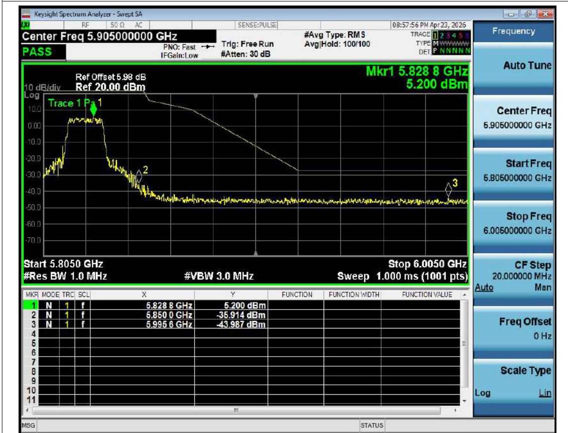
Band Edge NVNT a 5825MHz High Ant1
