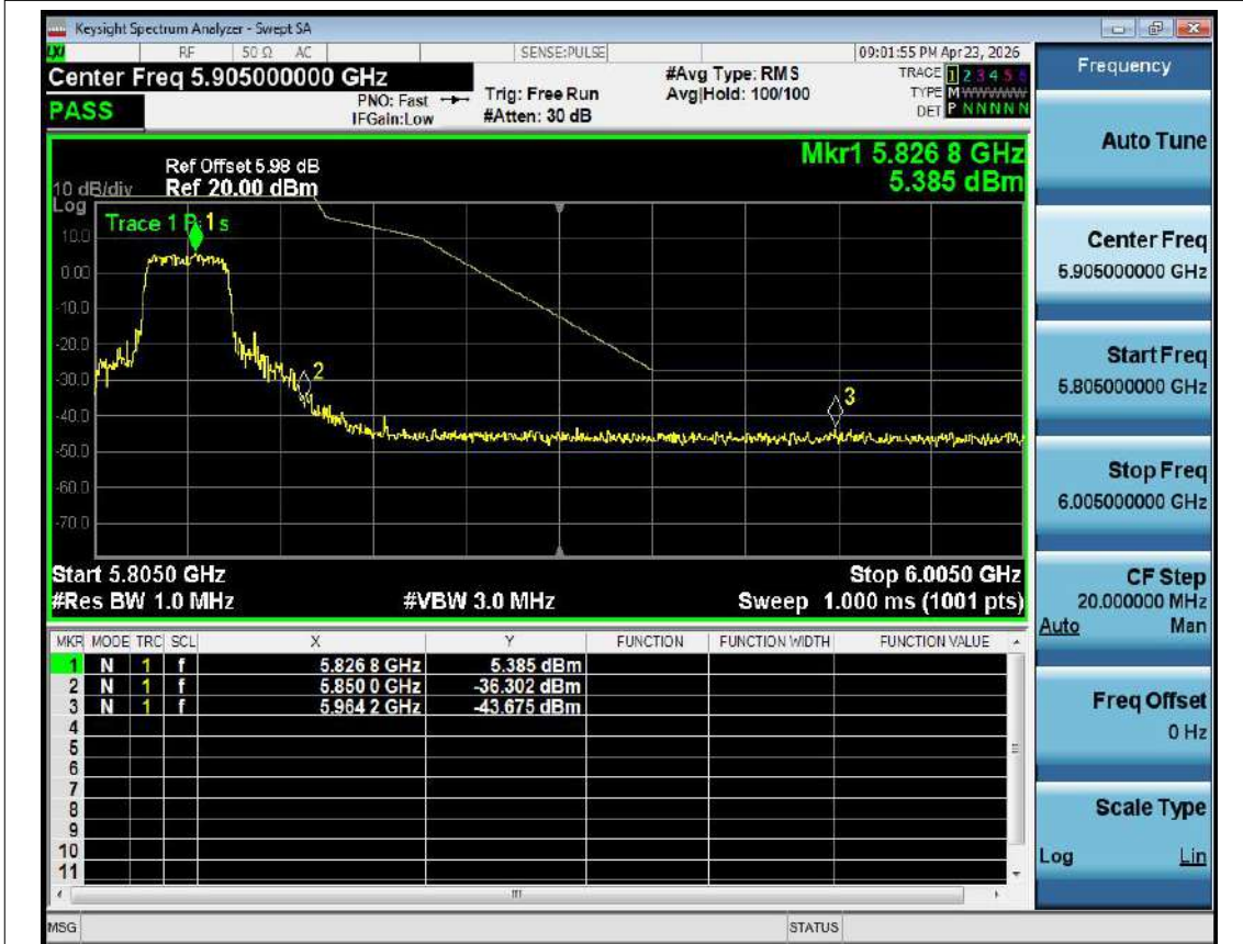
Band Edge NVNT n20 5825MHz High Ant1
