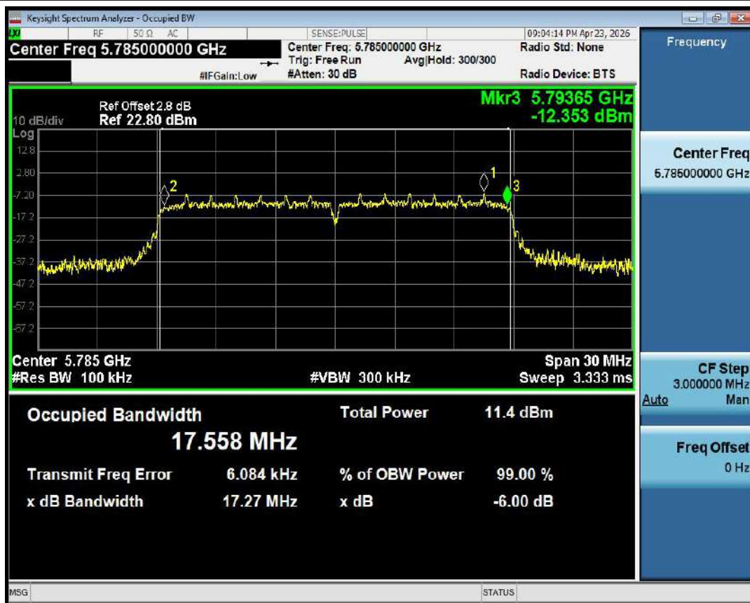
-6dB Bandwidth NVNT ac20 5785MHz Ant1
