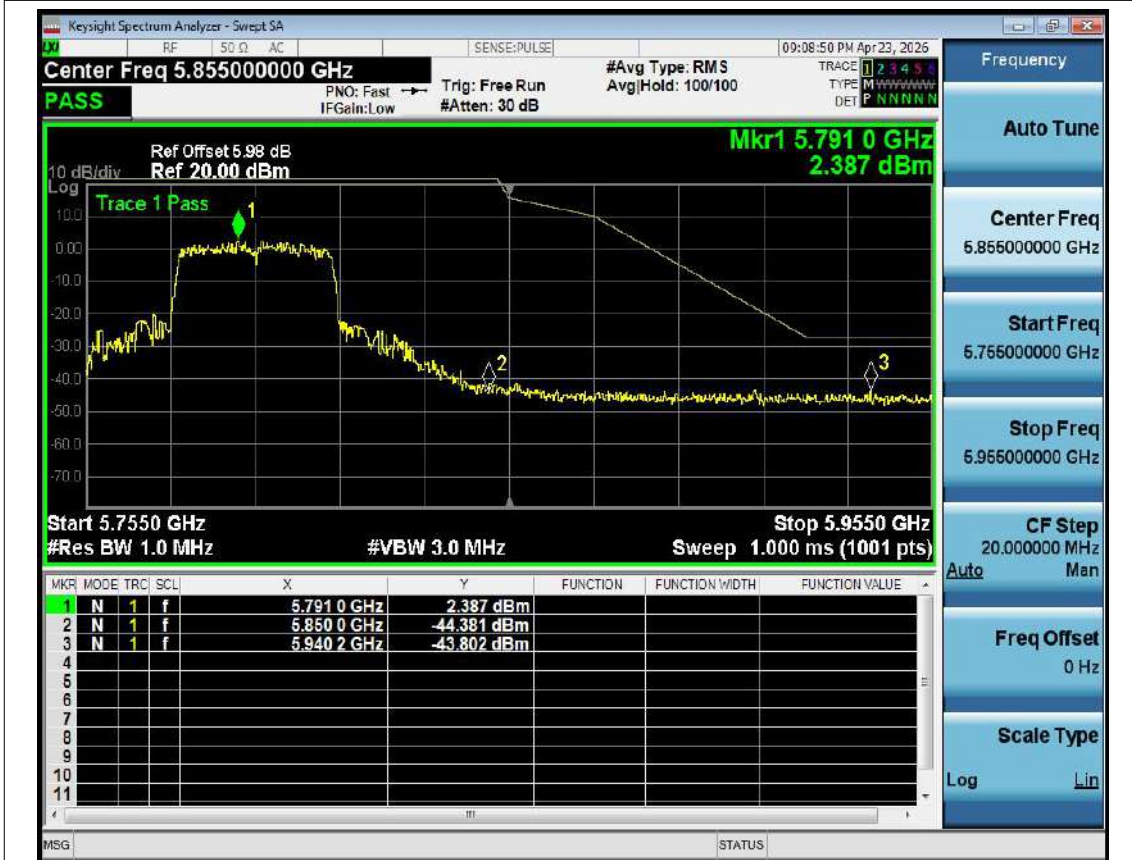
Band Edge NVNT n40 5795MHz High Ant1
